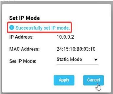
10. Now, ClearLink is fully configured to use the configured IP address/network settings you set above. ClearLink will use these settings from now on whenever it connects to a network. These settings are stored in non-volatile memory that is retained between power cycles.
