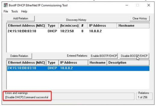
9. Now, ClearLink is fully configured to use the configured IP address/network settings you set above. ClearLink will use these settings from now on whenever it connects to a network. These settings are stored in non-volatile memory that is retained between power cycles.
