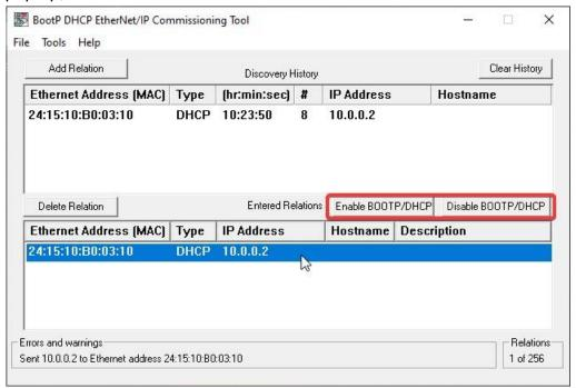
8. To ensure ClearLink uses the configured IP address upon startup, click "Disable BOOTP/DHCP". Verify that DHCP is disabled, by referencing the "Errors and warnings" section:
