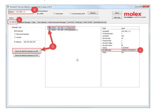
Note: If you do not see the ClearLink after clicking the "Send List Identity Request on UDP" ensure your network configuration includes a DHCP server (See <u>ClearLink Network Configuration</u> for valid network configurations). Some routers can be configured to block the UDP messaging so if you still experience issues you can look up the ClearLink's assigned IP address directly from the router/DHCP server and manually type in the IP address in the Station field.
