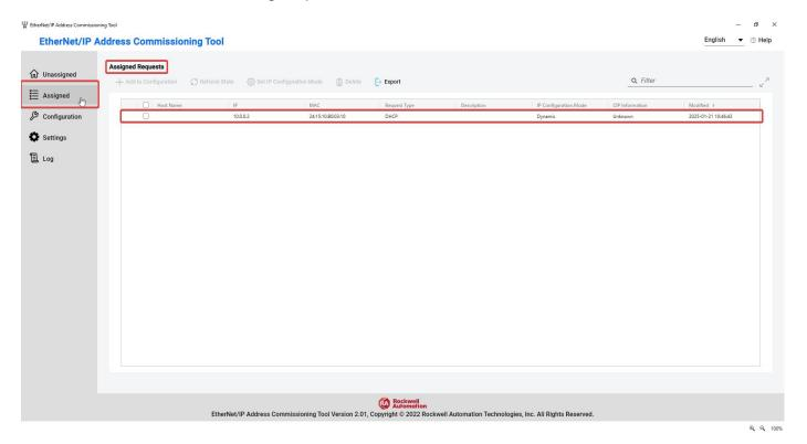
7. Select the row corresponding to ClearLink, then click the "Set IP Configuration Mode" button at the top.
